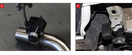
Once happy with fitment of Scorpion Exhaust, fully tighten up all clamps and fixing and plug in the electronic valve motors.
